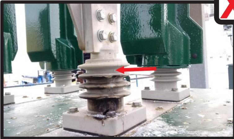
Hairline crack in insulator due to uneven torquing during bushing installation
